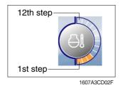
① This gauge indicates the temperature of coolant in 12 step gauge.
